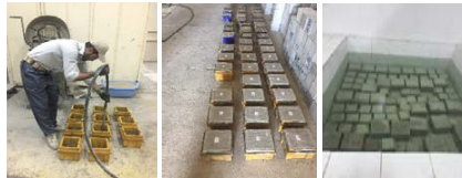
Figure 1. Dry and wet processes of test and curing specimens
