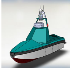
Figure 2. The proposed USV design for harbor surveying
