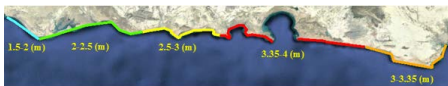
Figure4. Beach classification based on the maximum wave height at a point to a depth of 10 meters
