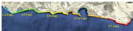
Figure5. Beach classification based on the maximum wave height at a point to a depth of 25 meters
