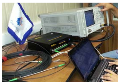
Figure 1. FBG sensors incorporated in the laboratory indoor test setup
