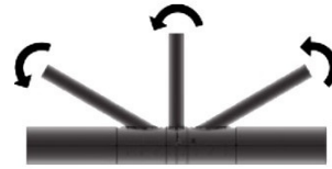
Figure 1. The considered in-plane bending (IPB) load case applied to KT-joints
