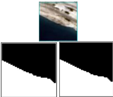
Figure 1. Top center image is selected coast from Landsat satellite. Classified images from left to right relative to SPSAM and MSPSAM with scale factor of 2.
