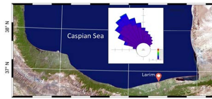
Figure 1. Wave rose at the project site location
