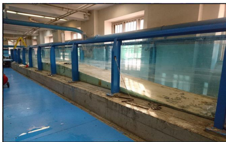
Figure 3. Wave flume University of Tehran
