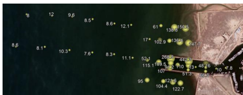
Figure 3. The location and average diameter (in micrometer) of the seabed samples in Deylam
