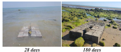
Figure 1. Placing the samples in tidal conditions to investigate SF's effectiveness on the characteristics of SWSSC after curing
