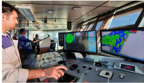
Figure 2. Display unit of EIT system at bridge of Khazar ship
