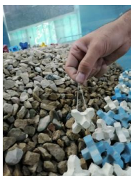
Figure 5. Proper placement of the armor layer in the laboratory
