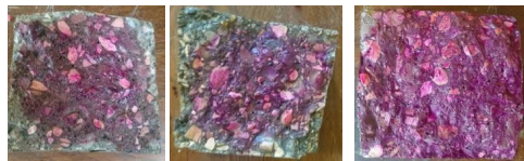
Figure 4. Comparing SW and FW on the carbonation depth and investigating the effectiveness of adding SF on accelerated carbonation depth of SWSSC results. The Left: reference concrete, Middle: SWSSC, Right: modified SWSSC with SF.
