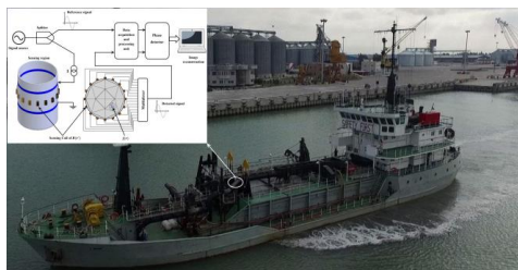
Figure 1. Dredger ship, Density-meter installation position.
