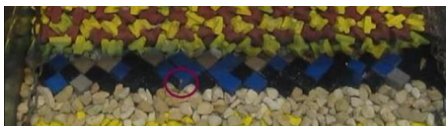
Figure 4. Toe layer consisting of three rows of cube2 with sacrificial rock- after the test of 1.2 times H_s
