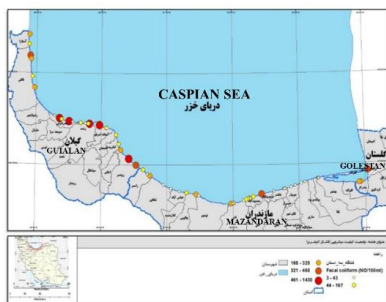
Figure2: Pollution map of swimming areas in the southern Caspian Sea (based on coliform fecal concentration)
