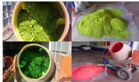
Fig. 1: Marking sand traces with four inks of yellow, orange, red and green, using sands from Amirabad Port coastal area
