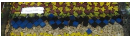
Figure 3. Toe layer consisting of three rows of cube1- after implementing the test of H_s
