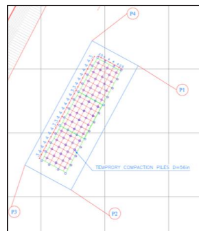
Figure 4. Vibration piles plan
