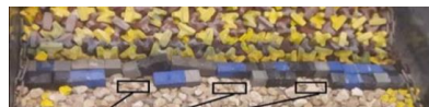
Figure 6. Toe layer consisting of cube2 (parallel) - after implementing the test of 1.2 times H_s
