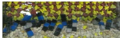
Figure 5. Toe layer consisting of cube2 (perpendicular) - after implementing the test of 1.2 times H_s
