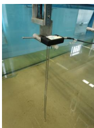
Figure 4. Resistance wave gauge sensors used in the laboratory to measure the wave height
