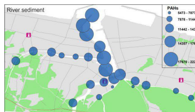
Figure2. Spatial distribution of the total concentration of PAH compounds in surface sediments (larger circles indicate higher concentrations of PAH compounds)
