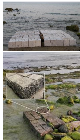
Figure 1. Placing the samples in tidal conditions to investigate SF's effectiveness on the characteristics of SWSSC after curing
