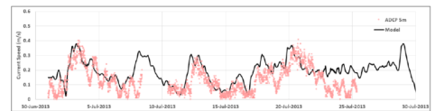
Figure 8. Comparison of modeling results of current speed with measured data (ADCP in depth=5m)
