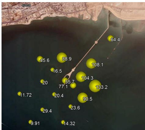
Figure 2. The location and average diameter (in micrometer) of the seabed samples in Nakhli Nakhoda
