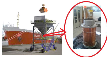
Figure 1. ECT system designed for solid mass flow measurement in ports.
