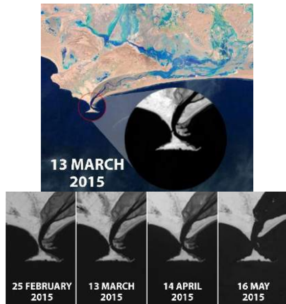
Figure 4. Breaching of the west bank (top), transition process (Bottom) [4]
