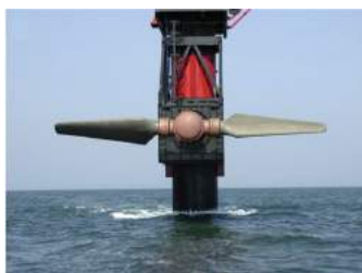
Figure 1. Horizontal axis marine current turbine [5].
