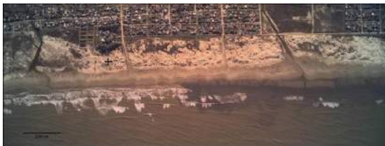
Figure 1: Surface waves attenuation by a small strip of muddy seabed (darker part of the sea from center to the right)
