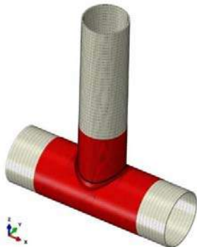
Figure 3. Numerical model of a FRP wrapped T-joint
