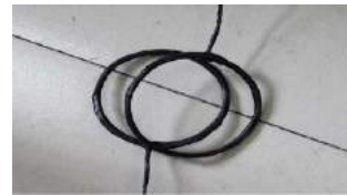
Figure4: the picture of the coupling coil
