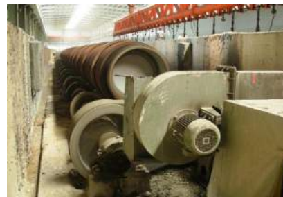
Figure 2. Piles under spinning process in the factory
