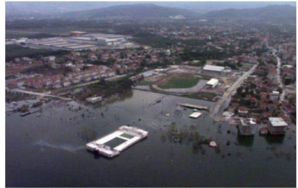
Figure 2. Subsidence at Golcuk along the southern shore of the Izmit Bay
