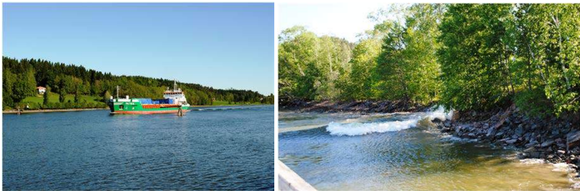
Fig. 1. Ship-generated waves in Göta River, Sweden; passage of ship Patria and observed drawdown.
